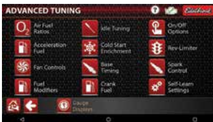
E-Tuner 4 app used for setup, calibration adjustments, engine system monitoring, and data logging.
